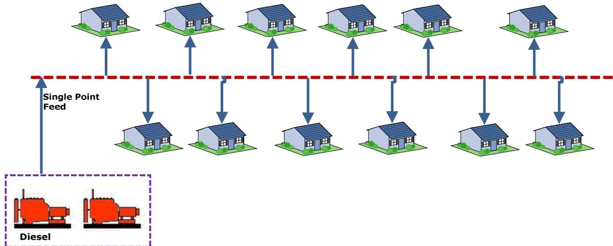
Putting Uncontrolled solar distributed along the system can work only if the penetration is low, but can cause stability problems if the penetration goes higher. Does not yield significant savings.
