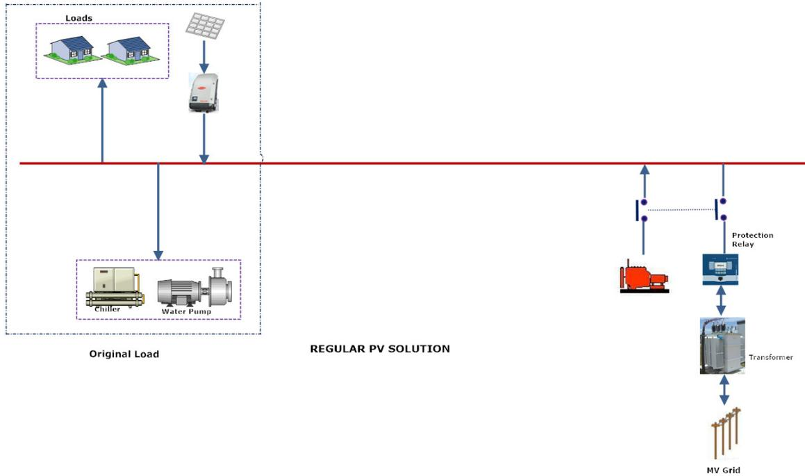
Later they want to expand their operation and decide to double the electrical load. The rural network does not have the capacity to supply the additional capacity and the network provider demands a very high cost for line upgrade. Just adding more solar is not going to solve the problem as even then it will not be possible to ensure that the power drawn will be within the line capacity, especially in view of the varying nature of the solar resource and the load.
