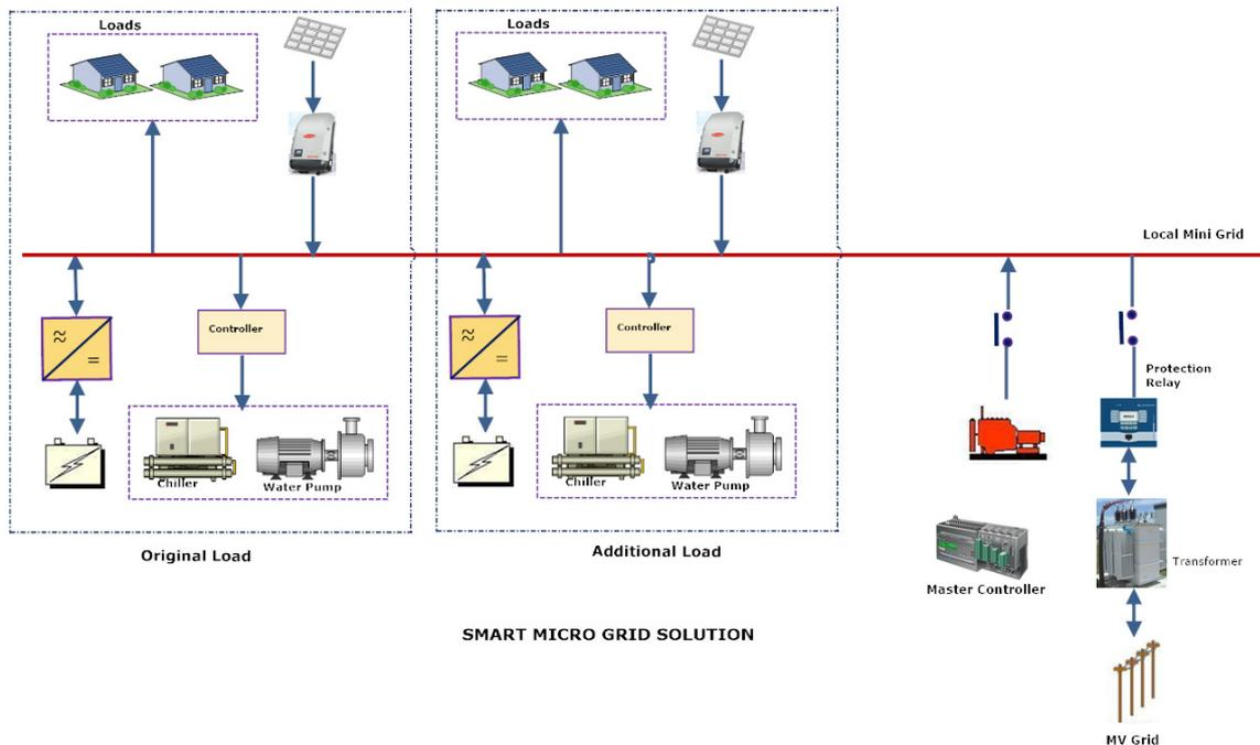
A Smart Microgrid can solve the problem by integrating the resources and managing the local network so that the additional load can be supplied without exceeding the line capacity. The costly line upgrade is avoided at a much smaller cost, while reducing the overall cost of electricity consumption.
