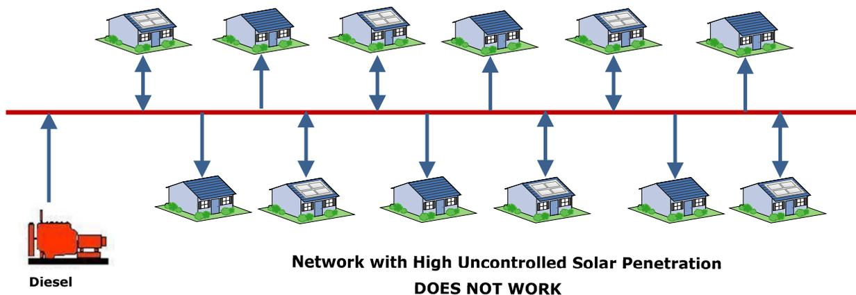
Penetration can be increased, even higher than 50%, with smart storage and Generation Management (The PV is ramped up/down at a controlled rate). Day time diesel consumption can be reduced significantly.
